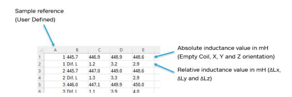
In all calculation files, only the absolute inductance values are used (empty coil Le and inductance values for each orientation Lx, Ly and Lz.
