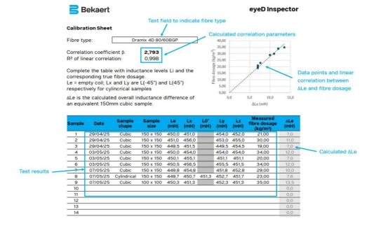
Note 1: The equivalent relative inductance  $\triangle$ Le is calculated as the sum of the three orthogonal measurements Li combined with the empty coil measurement, with a correction based on the sample shape and size. This approach allows the correlation to be independent of the sample shape and size.
