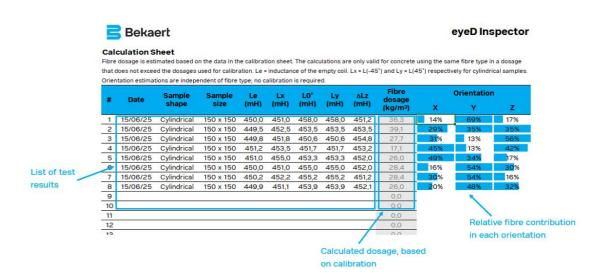
Note 1: The calibration is only reliable to be used for dosages that do not exceed those used during calibration. When the calculated dosage is higher than the dosages used during calibration (=extrapolating) consider adding extra test results in the "Calibration" tab.
